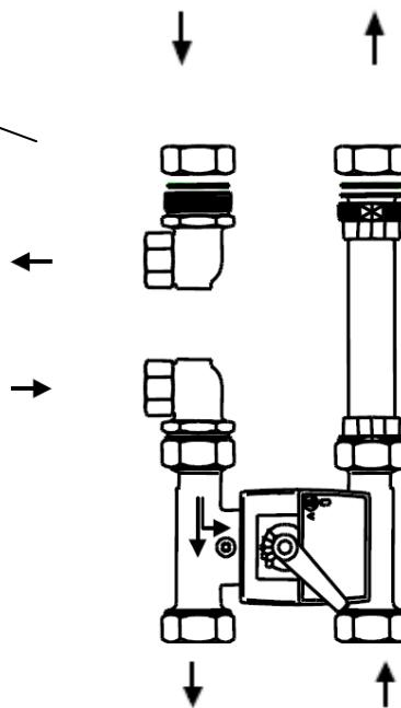
1 1/4" internal thread to alternative heat source (e.g. oil or gas boiler)
