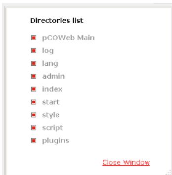
The "index" folder contains files where changes can be made to settings on the heat pump. No changes can be made to settings in all other folders.
