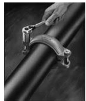
Once assembled, the Victaulic coupling meshes with the beads in the pipe. The pressure-reacting C-shaped seal adapts to the standard-roll or mill-grooved pipe. All supplied couplings come with a seal approved for domestic hot water systems (up to 110 °C).
