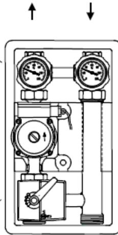
Ball valve return flow with blue thermometer and integrated gravity control:
